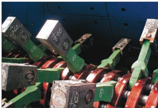
Rotor size 1600 mm dia. x 2800 mm width
