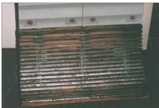
Impact wall furnished with grinding ledges and replaceable grate in the lower section for reducing oversized grain
